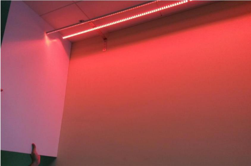
FIGURA 68 – PROFILI CON STRIP LED, PRIMO PROTOTIPO
