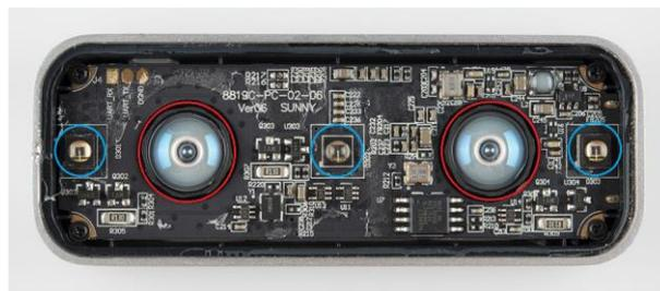
FIGURA 6 - L'INTERNO DEL LEAP MOTION: IN ROSSO SONO CERCHIATI I DUE SENSORI INFRAROSSO, IN AZZURRO I TRE EMETTITORI INFRAROSSO.
